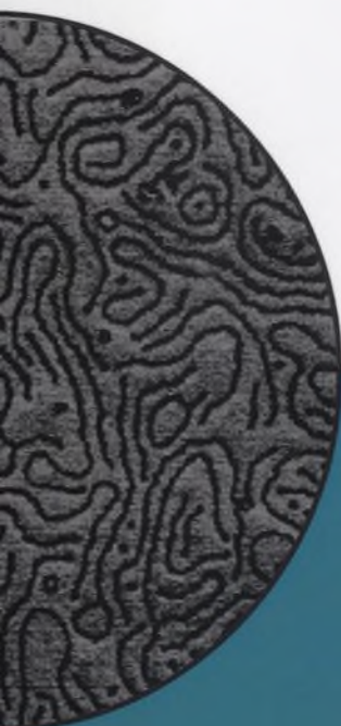
Cover illustration: Atomic force microscopy image of a thin block copolymer film in the process of ordering. Image courtesy of J. Howse.
